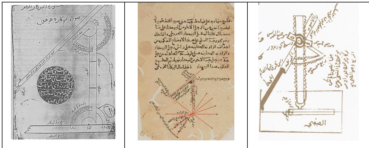
Figure 1: Examples of conic-section compasses in Arabic manuscripts, from left to right, (a) al-Qūhī (b) al-Siğzī, (c) Abu l-Qasim al-Asturlabi
