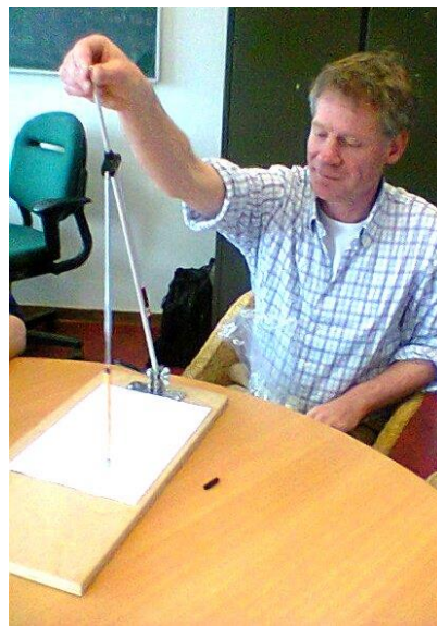
Figure 14: Henk Hietbrink and his home-made conic-section compass
